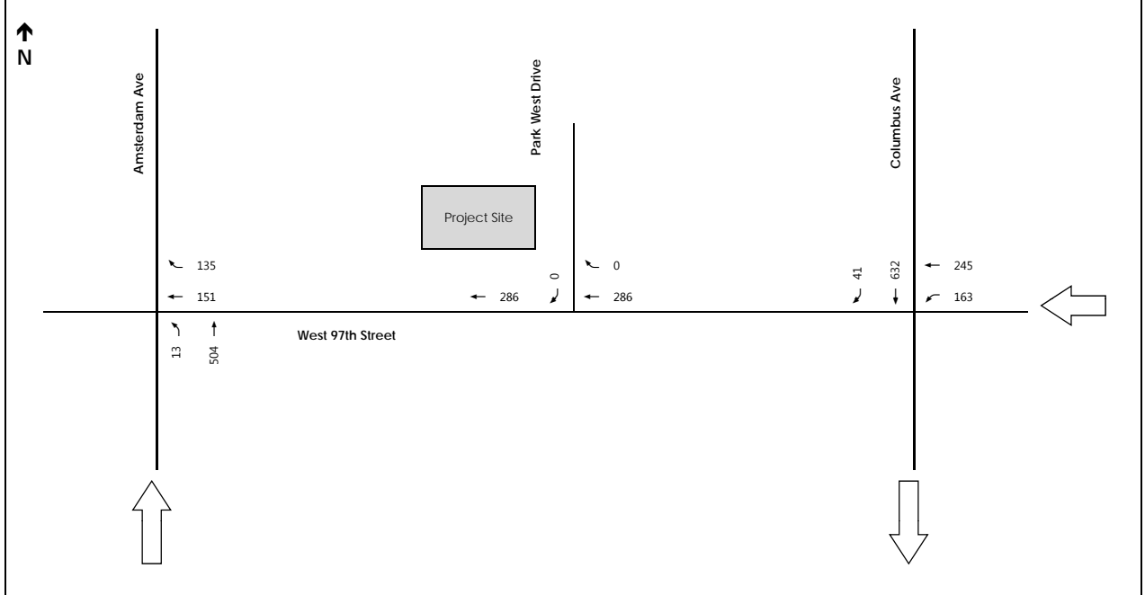
Construction a.m. Peak Hour (6:00 a.m. - 7:00 a.m.)
