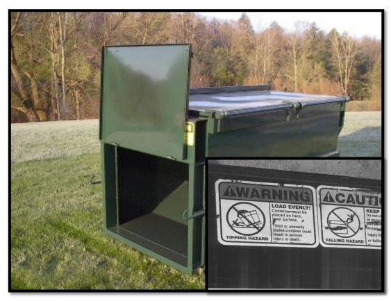
Photo 3. The two-yard steel compactor container and warning labels depicting crushing hazard. (Photo courtesy of OSHA)
