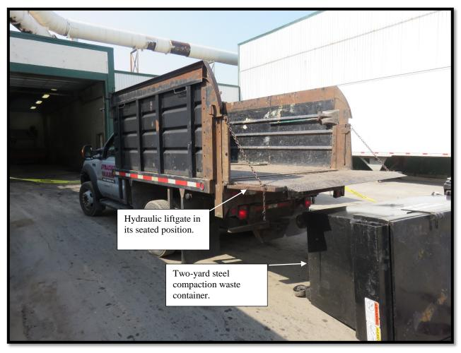
Photo 1. The truck with hydraulic liftgate being used to load and unload containers and the container after falling from the liftgate. (Photo courtesy of OSHA)
