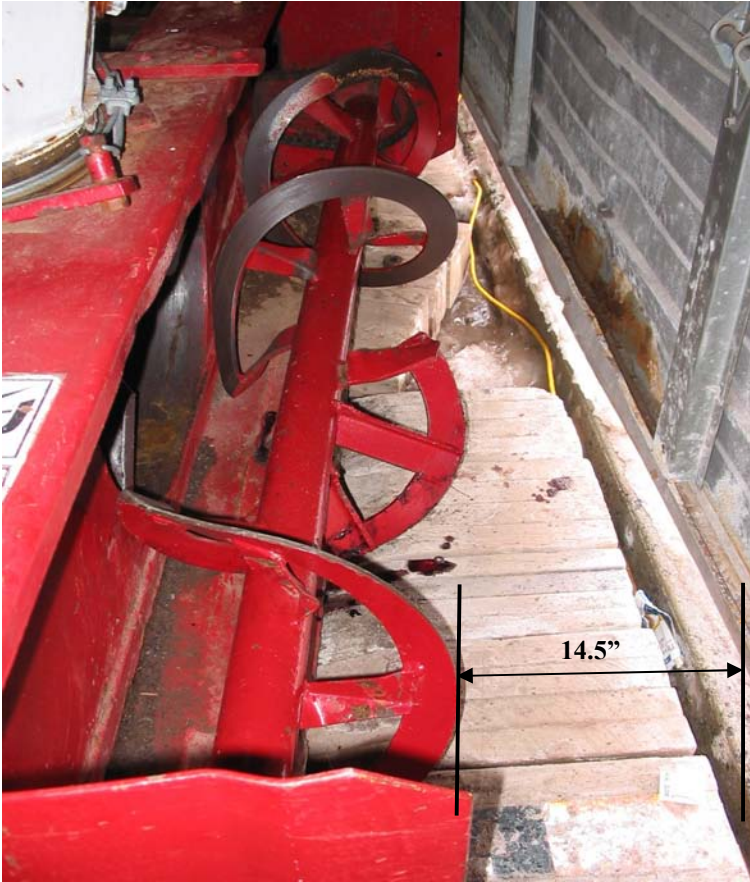
Photo 2. The victim was caught on the side where the clearance between the door and the rotating auger was 14.5 inches (Photo courtesy of OSHA).
