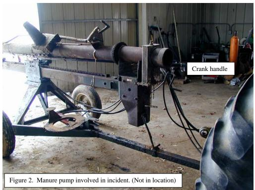
head near the rear connection to the PTO shaft. In standard practice, this crank is turned while the PTO is turned off so that the pump is not running.
