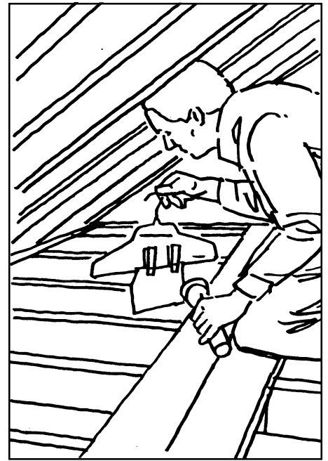
Fig. 10. Using a clothes hanger/plastic film combination to detect air leaks.
